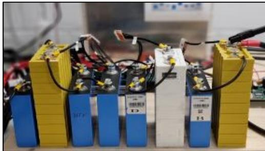
**Image 1:** A “patchwork battery” operated using ETA-Leveling: All cells are used and some have been stored for several years; the largest cell has a capacity of 68.6 Ah, the smallest of 45.9 Ah.
